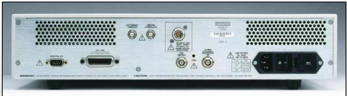
Figure 8. Rear panel of 2800 showing Type N input connector, external reference input, calibration output, external trigger and measurement complete BNC connectors, IEEE-488 connector, and DB9 digital I/O relay control lines connector.
